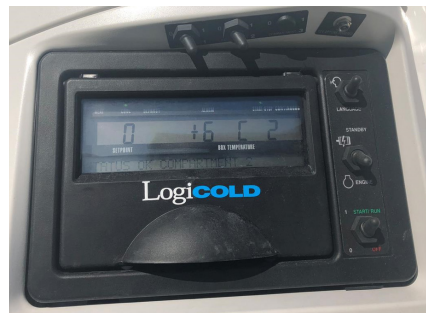
Carrier Vector 1950 Control Panel
