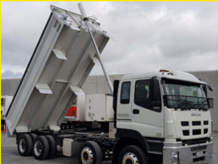
Large telescopic hydraulic cylinder to raise and lower a bin on a tipper.
