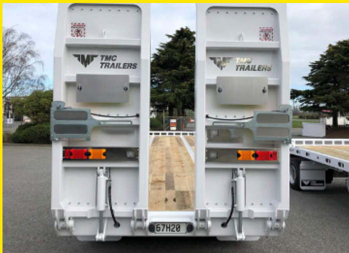
Two small rams fitted to raise the ramps.
