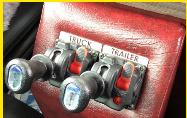
A typical control valve fitted to a tipper with the controls to raise and lower the bin on the truck and trailer.
