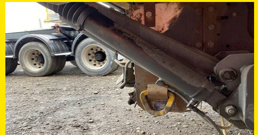
Hydraulic oil leaks, for example from the shaft seals or fittings.
