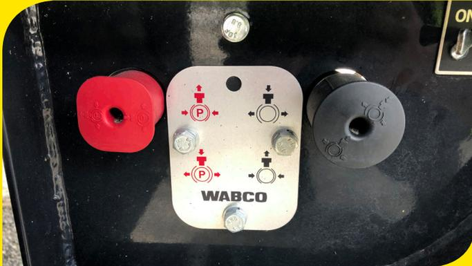
The Wabco PREV replaces the standard trailer park brake valve. It has two buttons, a black and a red. The main difference here is:
