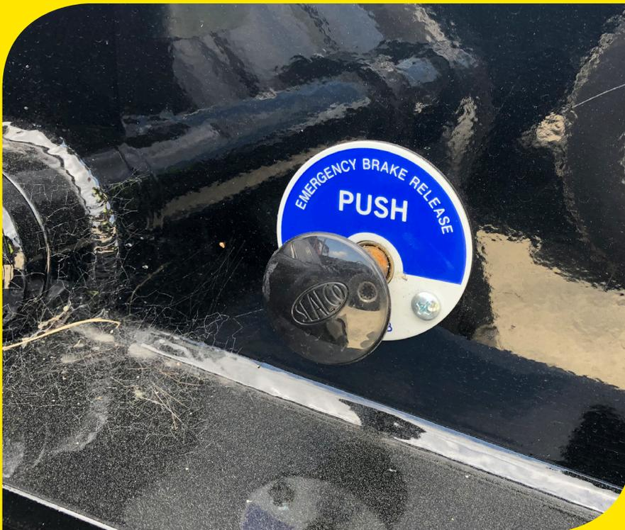
When the yard release valve is pressed-in, it would:
