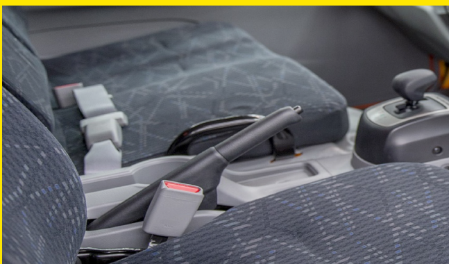
Typical handbrake lever of Cardon Shaft park brake equipped truck. You will notice the "ratchet" type feel.
