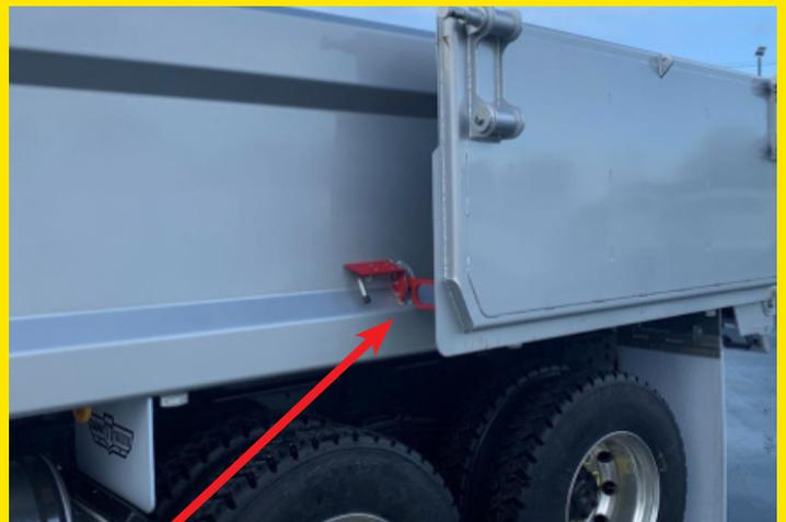
Swinging tail gate in the open position and securely locked with a latch.
