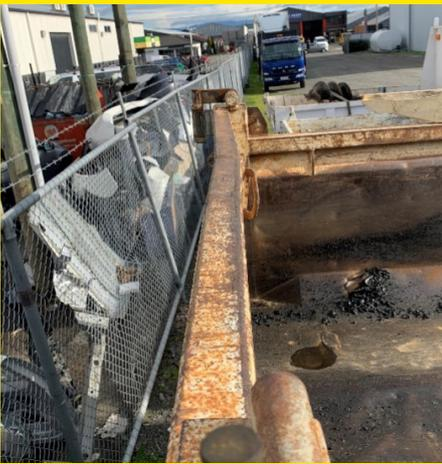
Bent tail door causing the tailgate to bind and not close properly.
