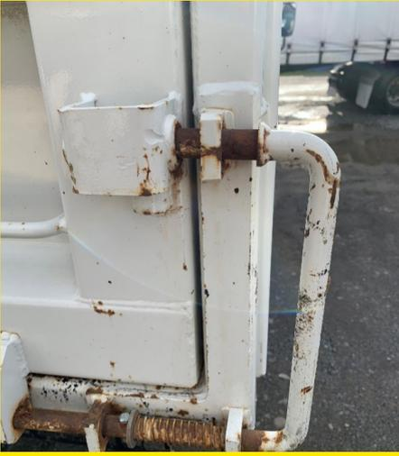
Tail door latch not engaging fully and appears bent. It has probably been kicked to get it to lock fully. This will be frustrating for the operator and potentially hazardous.
