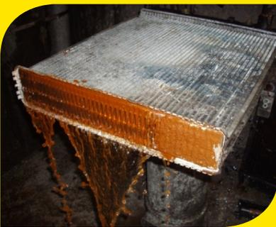
An example of a radiator that's had bad coolant and is being inspected at a radiator repair workshop.
