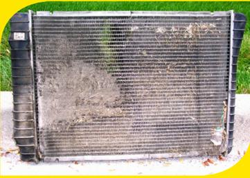
Here is an example of an engine radiator. In this case the radiator has been blocked to a level where it no longer cools properly because the air flow fins are blocked and in turn restricting the air flow to keep the coolant fluid to its
