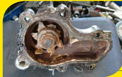
An example of a water pump that has been exposed to water turning to sludge and causing premature engine component failure.
