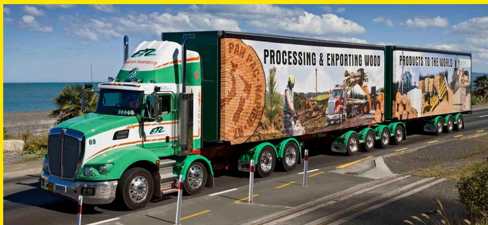
This is an example of a non-pro-forma unit that has been trialed in conjunction with the NZTA. It is carting pulp and timber between Pan Pac in Whirinaki and the Ports of Napier with a 62 ton gross.
