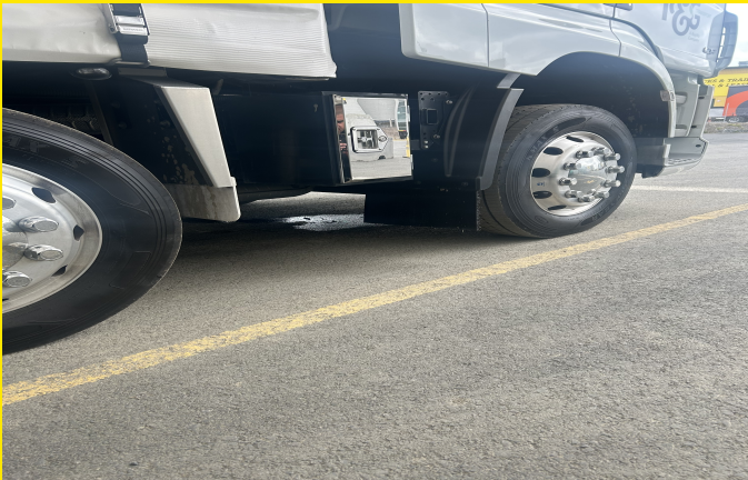
Notice a puddle under the cab after using the AC? This photo shows condensation that drains from the AC evaporator.
