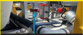
**Electro-Pneumatic Valves –** To control water flow from inside the cab.
