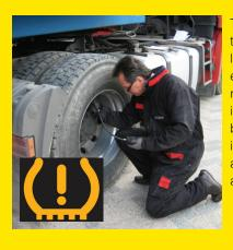
Tyre pressures are critical to maximising not just the life of the tyre but also fuel economy. Just a small reduction in pressure can increase fuel consumption by 5-10%. Most of the tyres in our fleet run pressures anywhere between 85 PSI and 115 PSI.
