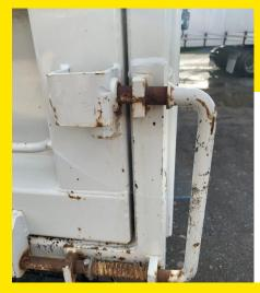
Tail door latch not engaging fully and appears bent. It has probably been kicked to get it to lock fully. This will be frustrating for the operator and potentially hazardous.
