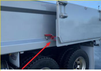
Swinging tail gate in the open position and securely locked with a latch.
