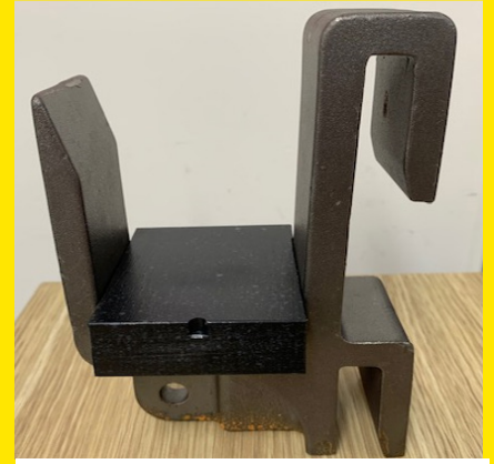
Mezz floor hook with a nylon wear pad in place.
