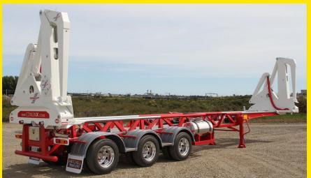
It is a common misconception that "Swinglift" and "side loader" are one and the same, but as you can see from the above, Swinglift is a brand with its own distinct characteristics. Swinglift is well known for its unique early chassis design, the lattice chassis. This design was developed to give a low tare weight while maintaining excellent strength.
