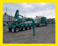
One key design characteristic is Swinglifts' unique lifting modules, which combine a leg over style stabiliser leg and lifting gibs all in one assembly. This means that deployment of the legs and lifting gibs happens quickly and efficiently with less moving parts.
