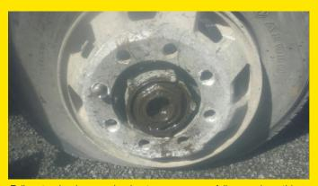
Failure to check your wheel nuts may mean a failure such as this.
