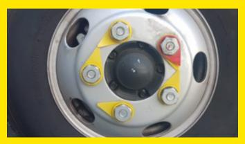
A red indicator over the top of a yellow indicator, or even on its own, indicates a wheel requires a retorque.
