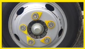
If there is a red wheel nut indicator on the outside of the yellow indicator then a retorque is required. Any misalignment of the wheel nut indicators also mean wheel nuts are potentially loose and must be checked
