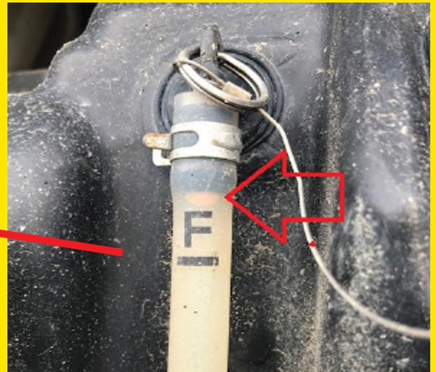
**These images show crystallised AdBlue that has formed after coming in contact with the atmosphere. You can see how this could cause blockages.**
