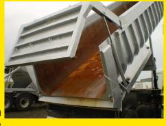
also makes it more difficult for material to stick to the floor, allowing for a cleaner dump cycle. However, the half-round has limitations when it comes to hauling equipment or pallets in the bed.
