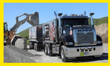
**Aluminium** is a great choice when carrying non-abrasive materials because of its lighter weight. It offers a greater payload capacity, as well as more protection from corrosion. On the flip side, aluminium is more expensive and its repair costs are greater than steel.
