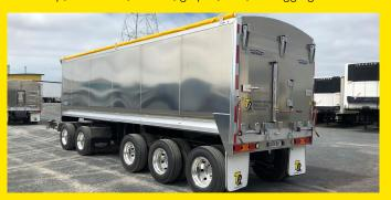
Being hydraulic powered, tippers require a bit more attention than your normal trailer. Always ensure that when connecting to a truck, the hydraulic connections are clean and free from dirt/debris and not damaged. Never leave hydraulic connections lying on the ground.
