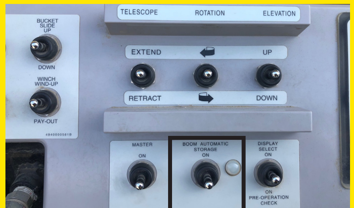
Aichi control panel showing auto stow switch.
