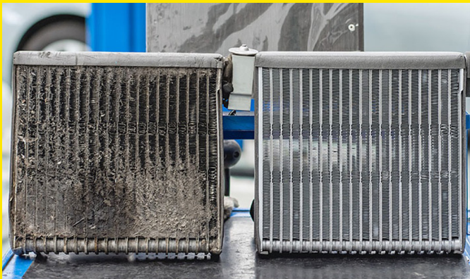
This image shows the difference between a clean and dirty evaporator.
