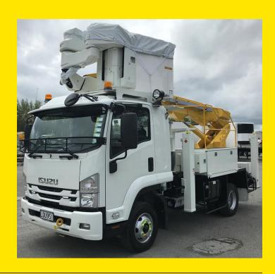
An EWP insulated boom has a non-conductive fibreglass section that must be extended to a minimum of 800mm before safe insulation from the steel section of the boom and the rest of the truck can be achieved. There is a minimum safe working extension mark on the fibreglass section. All live line work requires the boom to be extended to at least this distance.
