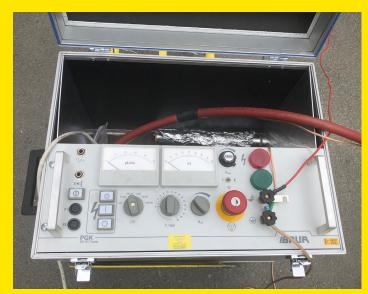
To test, the truck is raised off the ground and the extension leg feet are placed on insulated pads so that the truck is not grounded. The testing equipment used is a capacitor which can produce up to 100,000 volts. The capacitor is connected by a long cable to a suitable contact on the bucket.
