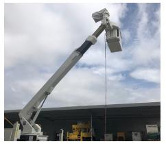
Voltage is gradually applied and the test equipment gauges are monitored for any sign of earthing between the insulated boom and bucket to the uninsulated boom and truck components. If after 3 minutes, at a minimum of 56,000 volts, there is no sign of leakage, the insulation can be declared safe and a passed test certificate will be issued and signed by a qualified electrical inspector.
