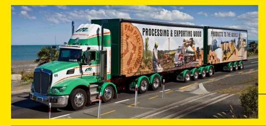
This is an example of a non-pro-forma unit that has been trialled in conjunction with the NZTA. It is carting pulp and timber between Pan Pac in Whirinaki and the Ports of Napier with a 62 ton gross.
