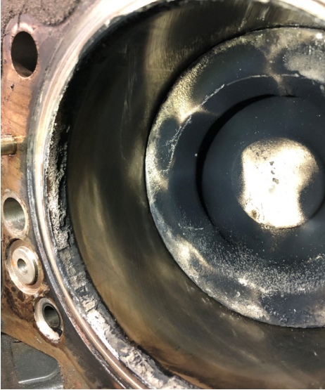
Below: Piston and liner damage attributed to excessive idle time.
