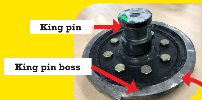
The king pin boss is welded to the skid plate and has failed (cracked) due to fatigue.
