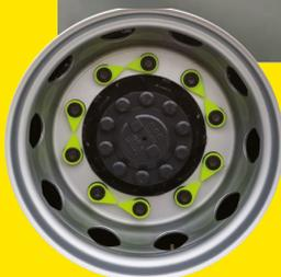
To prevent any wheel offs on TR Group vehicles we have been fitting the standard wheel nut indicators. These are the industry standard. With these you cannot see the wheel nuts coming loose at 90kph. (These are a visual indicator only.)
