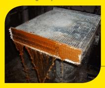
An example of a radiator that's had bad coolant and is being inspected at a radiator repair workshop.
