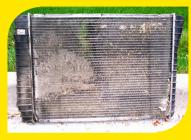
Here is an example of an engine radiator. In this case the radiator has been blocked to a level where it no longer cools properly because the air flow fins are blocked and in turn restricting the air flow to keep the coolant fluid to its
