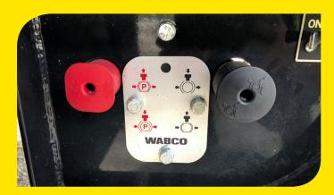
The PREV system parks on all axles by applying air pressure to all brake pots. These will stay like that until the air runs out or it is hooked back up to the truck.
