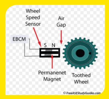
The wheel speed sensor and toothed wheel (otherwise known as the pulse wheel) work together to send signals to the eRoad unit. Generally, if a wheel bearing is out of adjustment or the sensor is loose in its mount, a greater air gap is created causing a fault. If this system faults it will default to GPS for speed. Wheel speed is a much more accurate speed pick up. This fault will bring up the blue status light. Please contact your local supplier for inspection.
