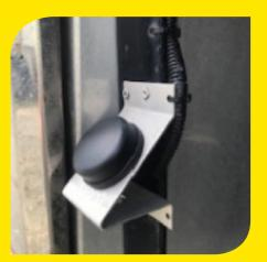
If the GPS beacon on the trailer is damaged or faulty, the system will not track the vehicle's position.
