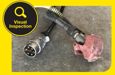
For trailers with eRoad, Pin 5 in the standard 7 Pin trailer connector must have a constant power feed to charge the battery in the eRoad unit. A common fault is the power fuse blows or has a bad electric connection eg. from the suzy lead.
