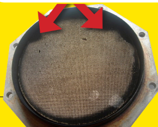
Partially Blocked DPD Filter
