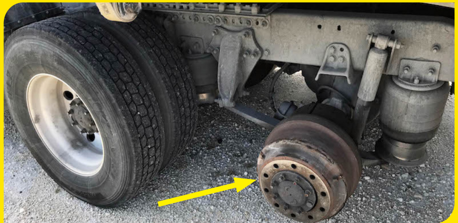
This is the end result of when a retorque is not completed. Our systems are designed to prevent this.
