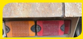
Damaged lights need to be replaced before travelling.
