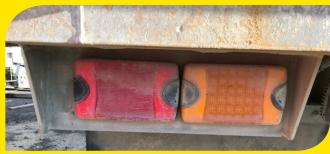
The above picture shows a missing reflector on the left side, this is easily lost and has a big impact on road side inspections.
