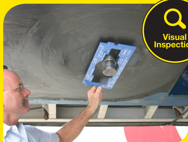
Inspecting kingpin shoulder and neck in wear limits.
