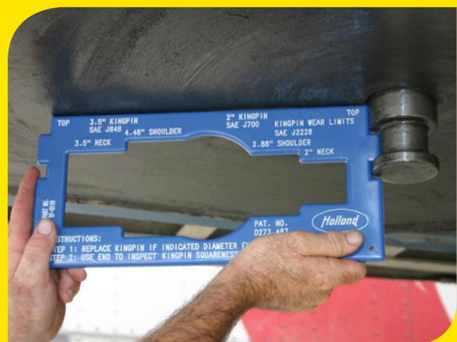
Inspecting kingpin squareness to skid plate.
