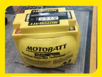
A swollen casing is a sure sign of a failing battery.
